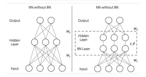
A new layer is added so the gradient can "see" the normalization and make adjustments if needed.
