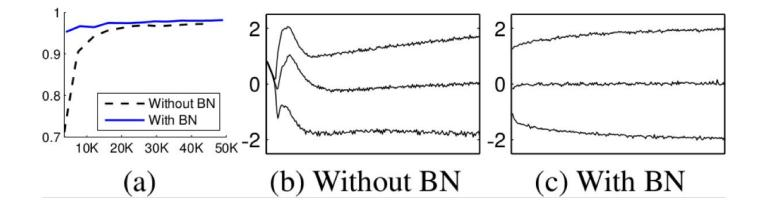
BN applied to MNIST (a), and activations of a randomly selected neuron over time (b, c), where the middle line is the median activation, the top line is the 15th percentile and the bottom line is the 85th percentile.
