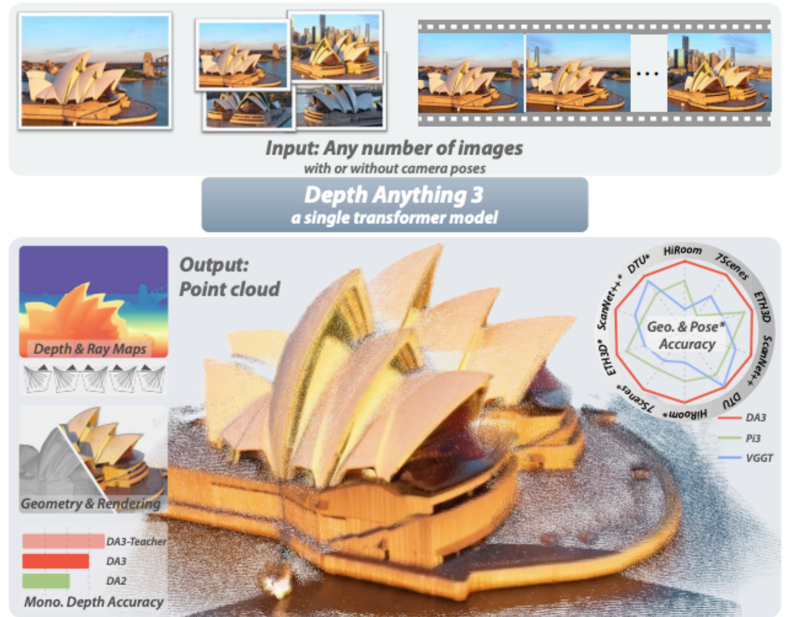
Figure 1 Given any number of images and optional camera poses, Depth Anything 3 reconstructs the visual space, producing consistent depth and ray maps that can be fused into accurate point clouds, resulting in high-fidelity 3D Gaussians and geometry. It significantly outperforms VGGT in multi-view geometry and pose accuracy; with monocular inputs, it also surpasses Depth Anything 2 while matching its detail and robustness.
