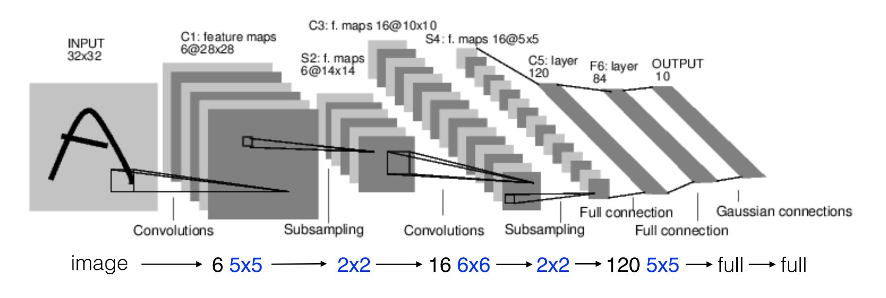
C5: Convolutional layer with 120 outputs of size 1x1 Each unit in C5 is connected to all inputs in S4 Number of parameters: (16x5x5+1)\*120 = 48120
