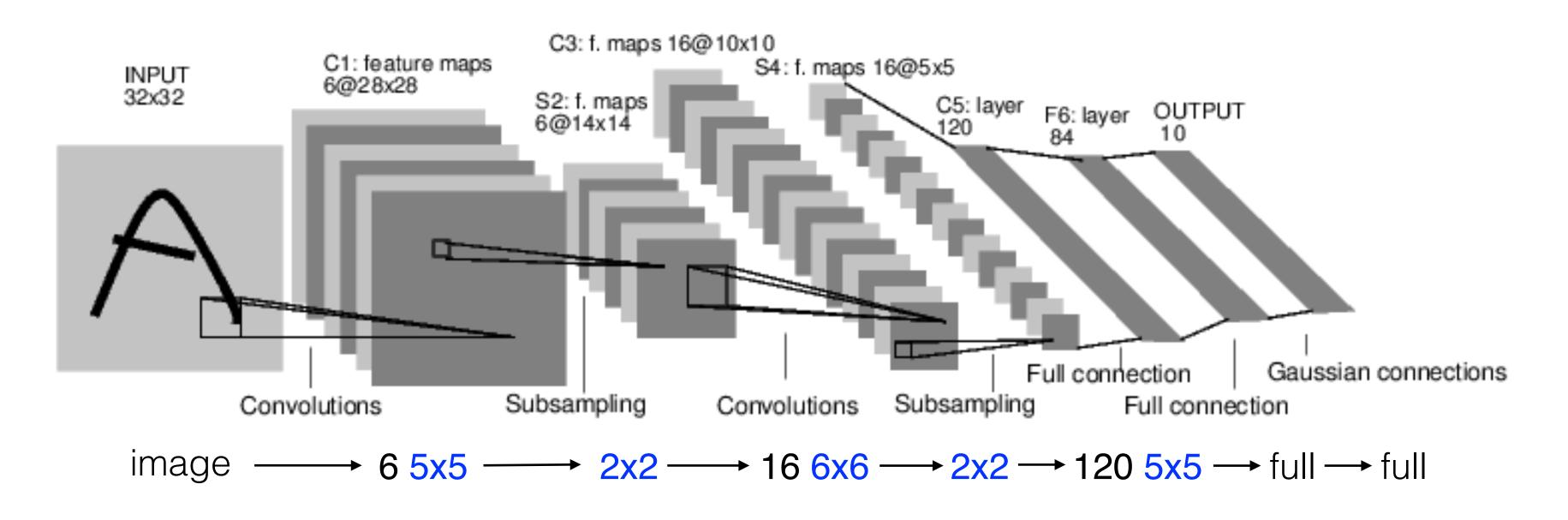
C1: Convolutional layer with 6 filters of size 5x5 Output: 6x28x28 Number of parameters:  $(5x5+1)^*6 = 156$ Connections: (5x5+1)x(6x28x28) = 122304Connections in a fully connected network: (32x32+1)x(6X28x28)
