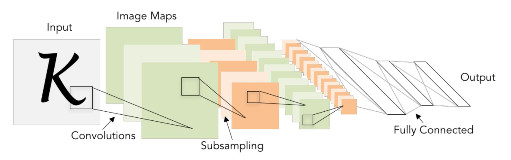
Applied backprop algorithm to a Neocognitron-like architecture Learned to recognize handwritten digits Very similar to our modern convolutional networks!
