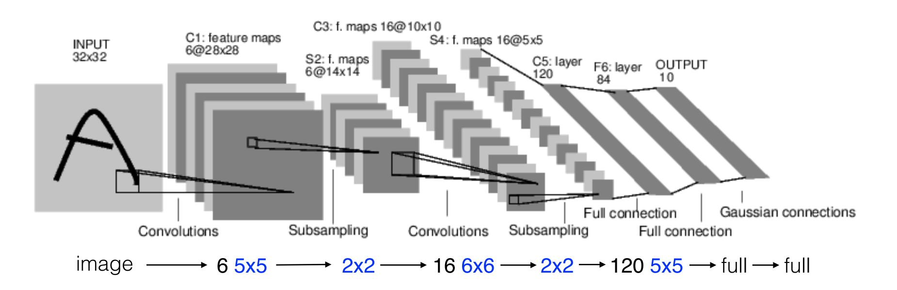
C3: Convolutional layer with 16 filters of size 6x6 Each is connected to a subset: Number of parameters: 1,516 Number of connections: 151,600 Output: 16x10x10
